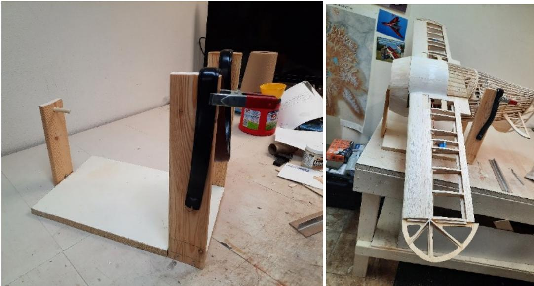
I'm always looking for tools to work smarter. I found a contouring gauge that is perfect for copying the top surface a wing in order to build the fuselage wing saddle.
