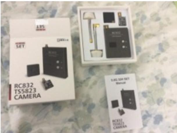
with the operator. On the model is the camera, the video transmitter. Power is supplied by a dedicated pack, or more commonly, using the flight battery through the balance lead. On the ground is the video receiver and the monitor or goggles. Both are generally powered with a single LiPo battery.
